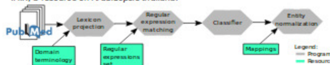
Fig. 2: Chained execution of TDM tools including the trained classifier predicts named-entities and relations on a relevant corpus (5000 abstracts).
